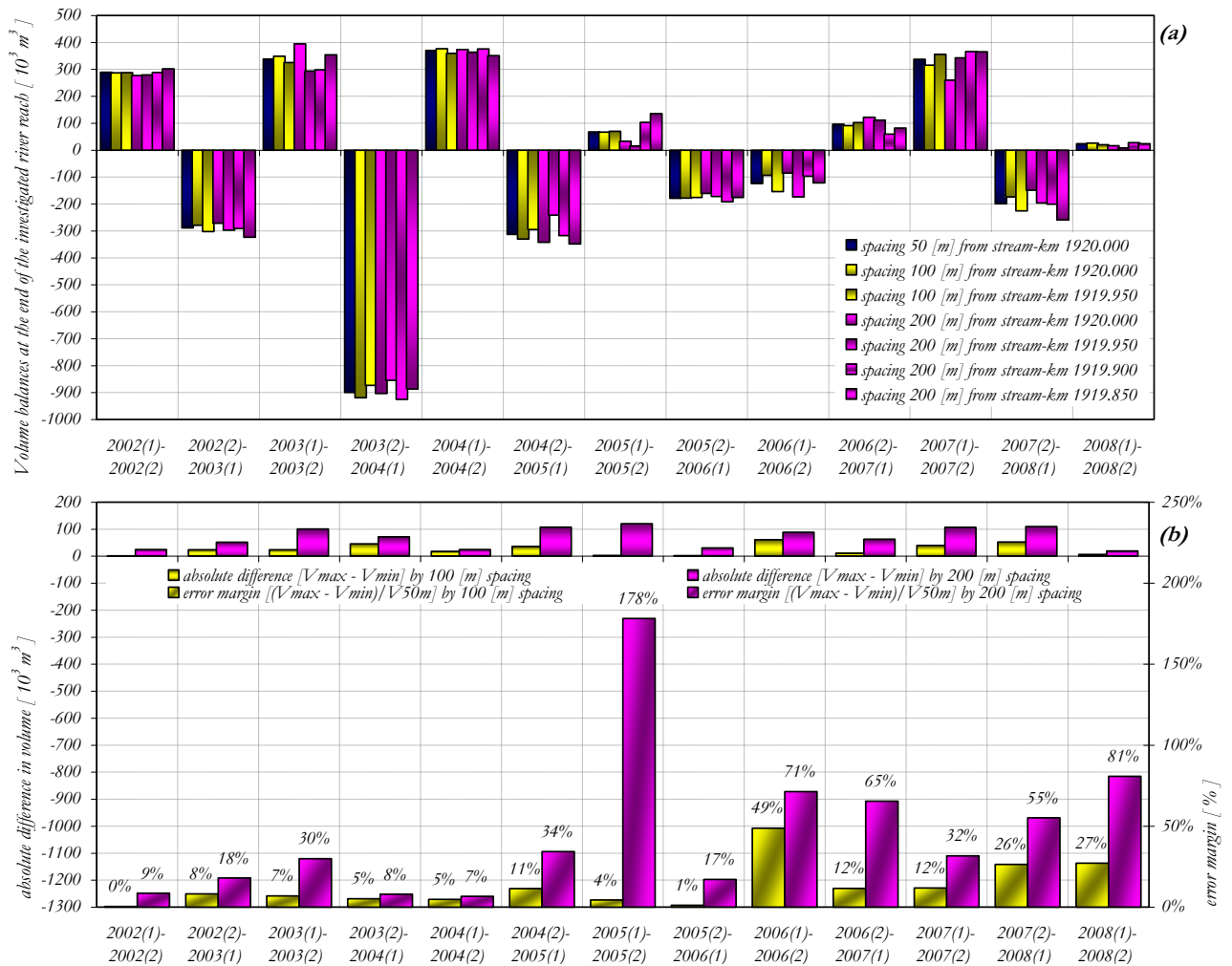
Figure 6.9: Sensitivity analysis on various longitudinal profile spacings: (a) volume balances at the end of the investigated river reach & (b) absolute volume differences by various spacings and the corresponding error margins
