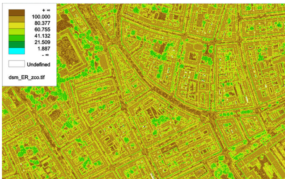
Figure 11: Echo ratio map of the test area: The numbers in the legend are assigned to the lower threshold of the classes. That means for the class that is visualized in dark green: The range of this class is 1.887 until 21.508. 21.509 is the lower threshold of the next class.
