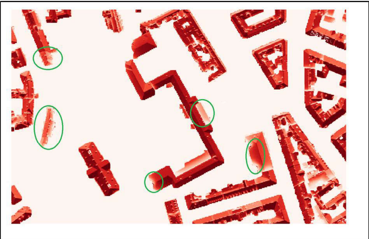
Figure 20: Solar irradiation map with the influence of objects outside of the rooftop area
