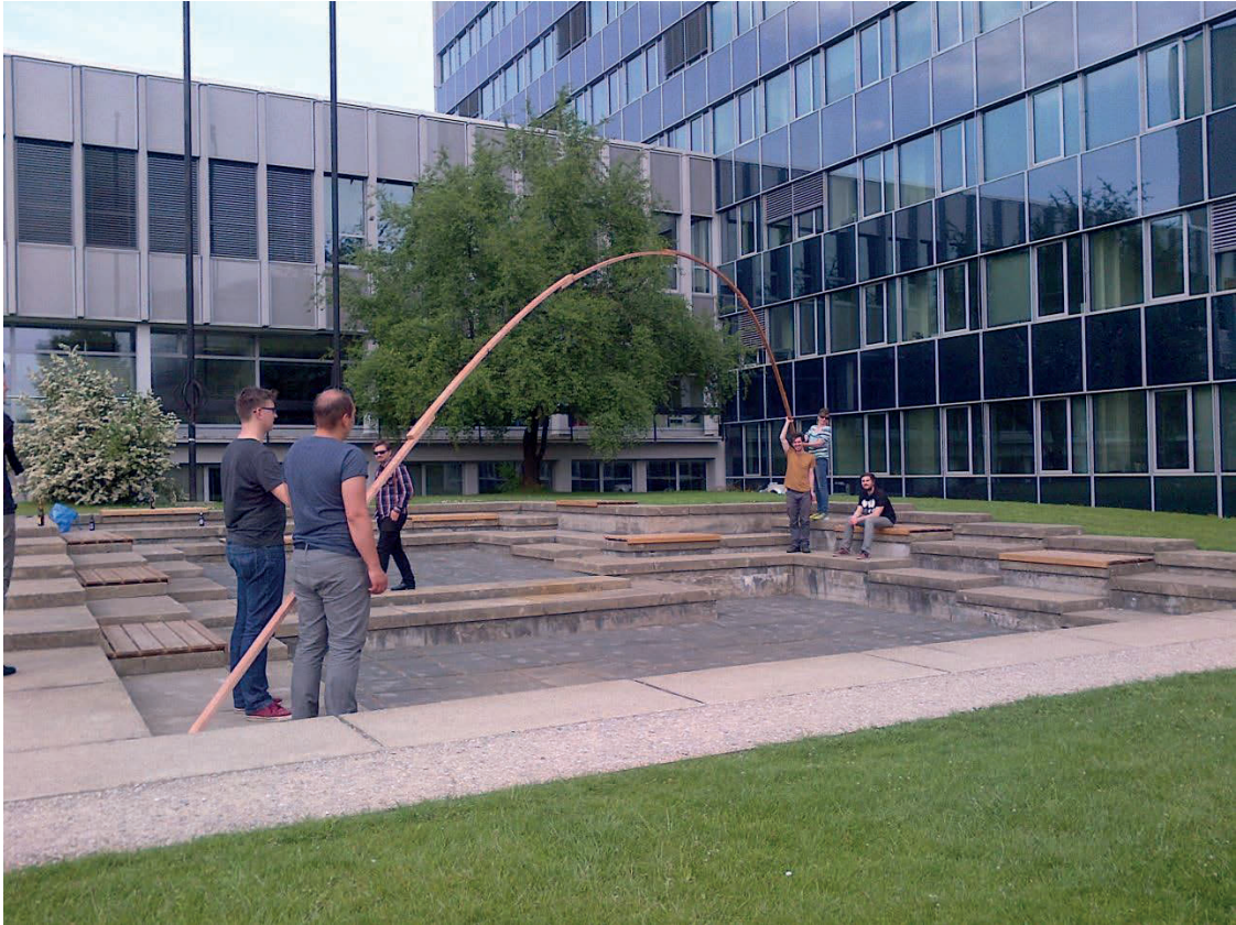
Fig. 4.13 Timber bending test [by author]
