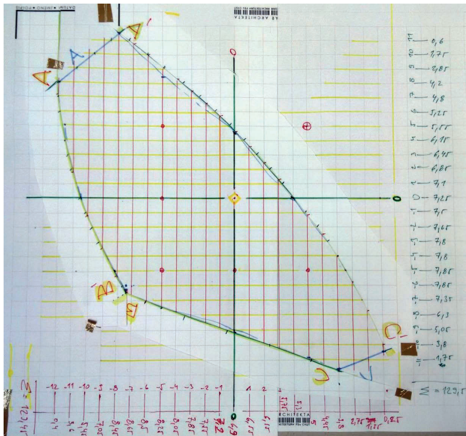
Fig. 4.8 Basic mesh top view from hanging chain form finding [by author]
