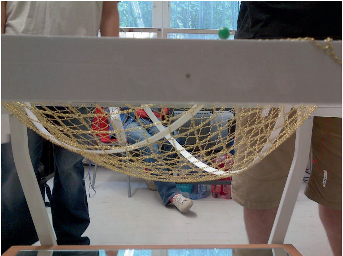
Fig. 2.15 Hanging chain model – Most precise physical design technology [by author]
