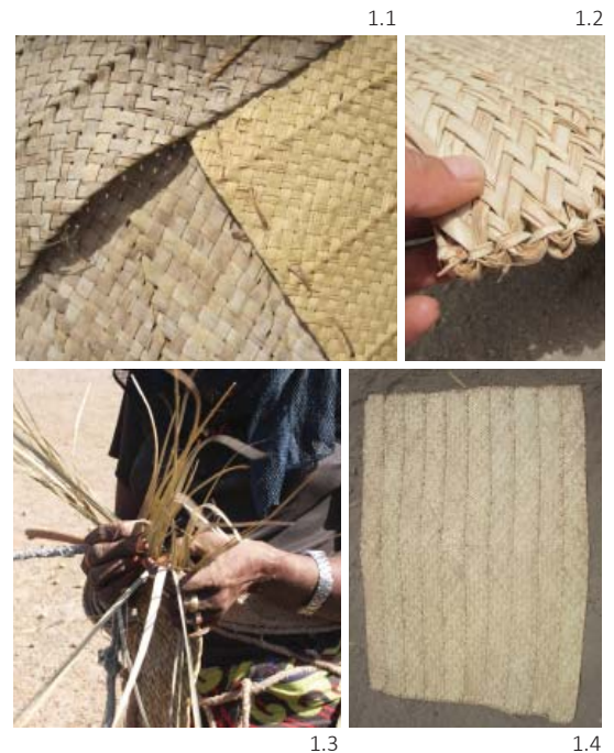
1.1 Different types of mats 1.2 Edge details 1.3 Afar woman weaving a mat 1.4 Type of mat that will be used for construction
