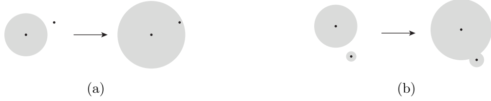
Figure 2.5: Two different types of nuclei growth restrictions: ingestion (a), coalescence (b) Black dots represent nucleation sites, gray areas the build up phase.
