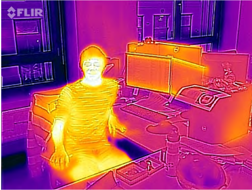
Figure 1.4: Infrared image taken with the FLIR ONE™ thermal imaging camera.
