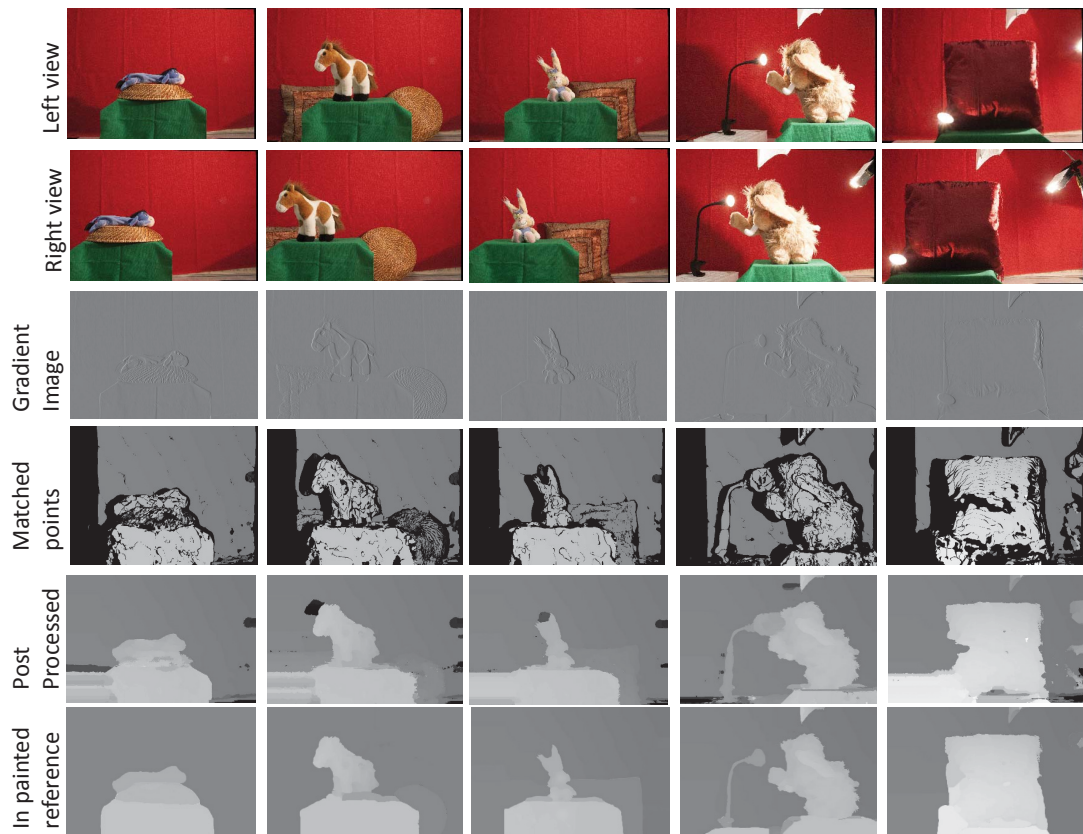
Figure 5.2: HDR stereo data set and their corresponding reference disparity maps. First two rows: the left and right views of the images, Third row: the gradient images corresponding to the left view, Forth row: the matched points from two views using the customized HDR cost-volume stereo matcher, Fifth row: the post processed disparity maps and, the last row: the in painted reference disparity maps.
