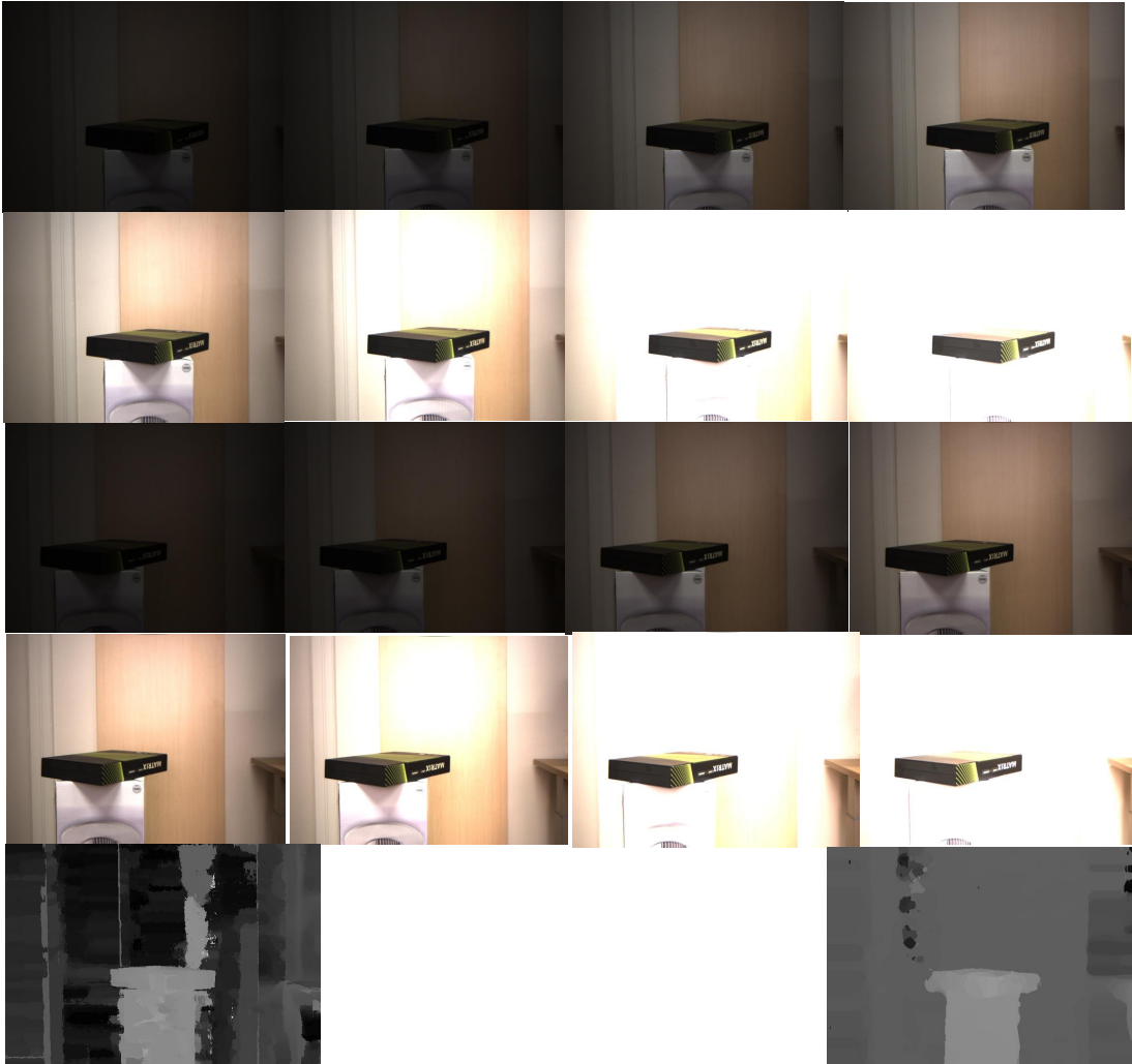
Figure 3.8: A complete LDR sample from our multi-exposed stereo data set captured with Bumblebee stereo camera. First and second row: left view, third and fourth row: right view, fifth row, left to right: LDR and HDR disparity maps. Exposure times from left to right (shown in two rows): 1/1024s , 1/512s , 1/256s , 1/128s , 1/64s , 1/32s , 1/16s and 1/8s . Baseline: 227 mm. LDR disparity map is computed using the middle exposure, 1/64s .
