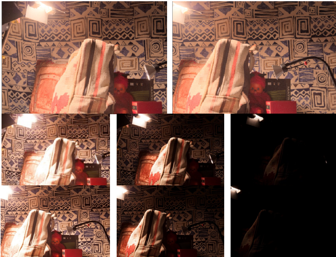
Figure 3.4: Stereo HDR data set example. First row: left and right views of an HDR pair (tone mapped using Drago TMO [DMAC03] for better display) with a baseline of 150 mm and dynamic range of 8140:1. Second row: left view in the highest, middle and lowest exposures (1/15s, 1/250s, 1/2000s). Third row: same as the second row for the right view.
