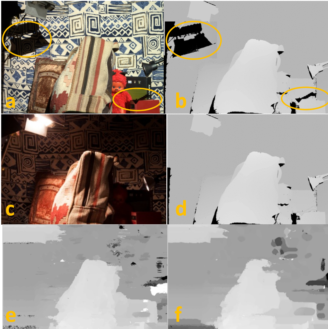
Figure 4.6: Reference disparity map computation. (a): Full projected scene, with non-illuminated regions (shadows are marked black) specified; (b): computed reference map before manual post processing (shadow holes); (c): left LDR mid-exposed image; (d): calculated reference disparity after post processing; (e): LDR stereo matching result corresponding to (c); (f): tone mapped stereo matching result corresponding to top row of Fig. 3.4.
