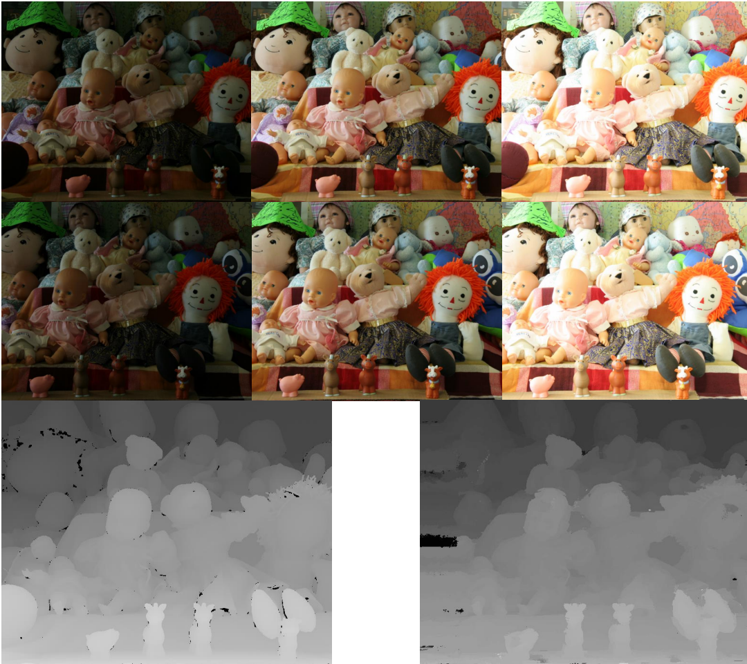
Figure 3.6: A complete LDR sample from the Middlebury multi-exposed stereo data set [HS07]. First row: left view, second row: right view, third row, left to right: LDR and HDR disparity maps. Exposure times from left to right: 1/4000s , 1/1000s and 1/250s . Baseline: 160 mm, between views 1 and 5 of Middlebury dataset. LDR disparity map is computed using the middle exposure, 1/1000s .
