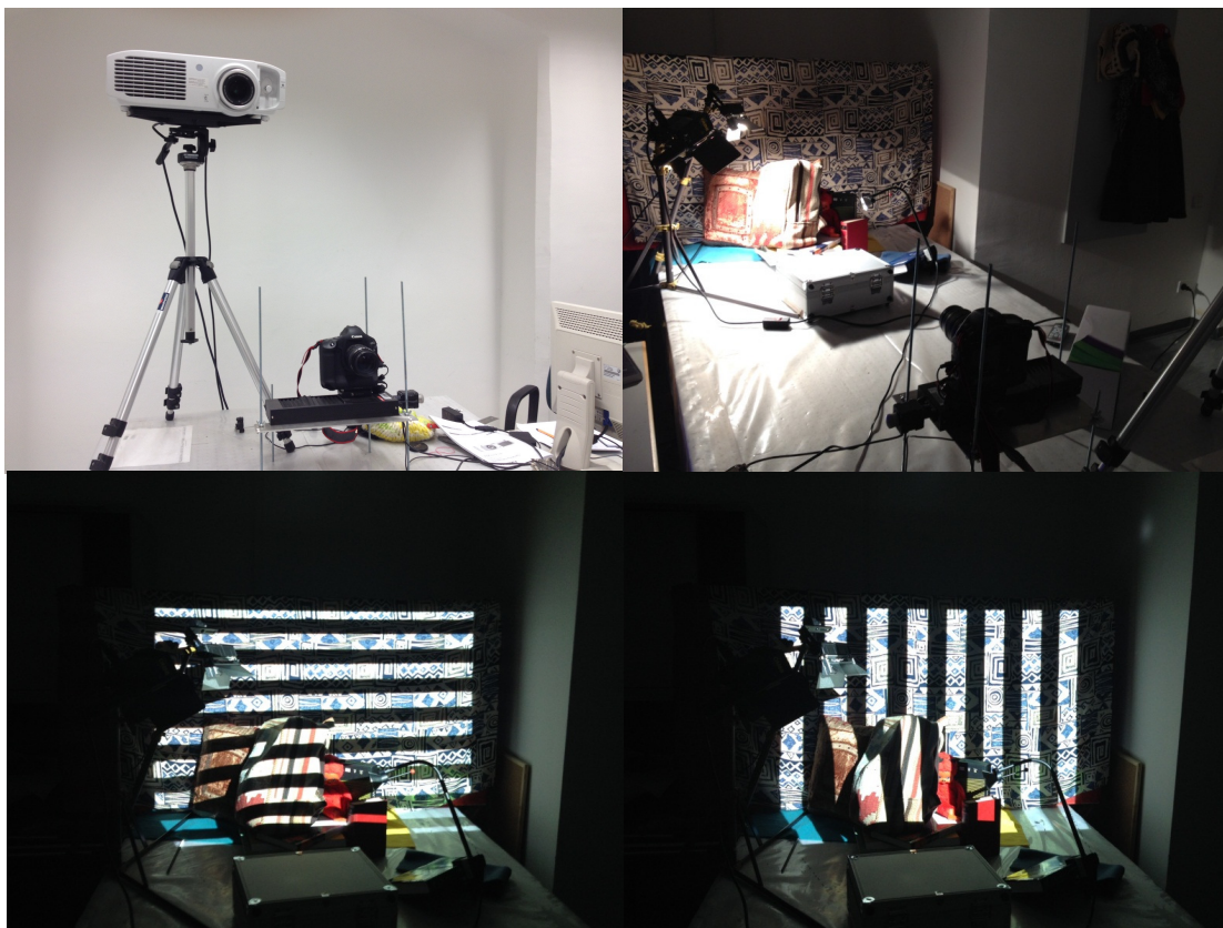
Figure 4.4: Scene capturing process. Top left: experimental setup, top right: HDR image capturing, bottom left: example of a horizontal Gray-code image, bottom right: example of a vertical Gray-code image.
