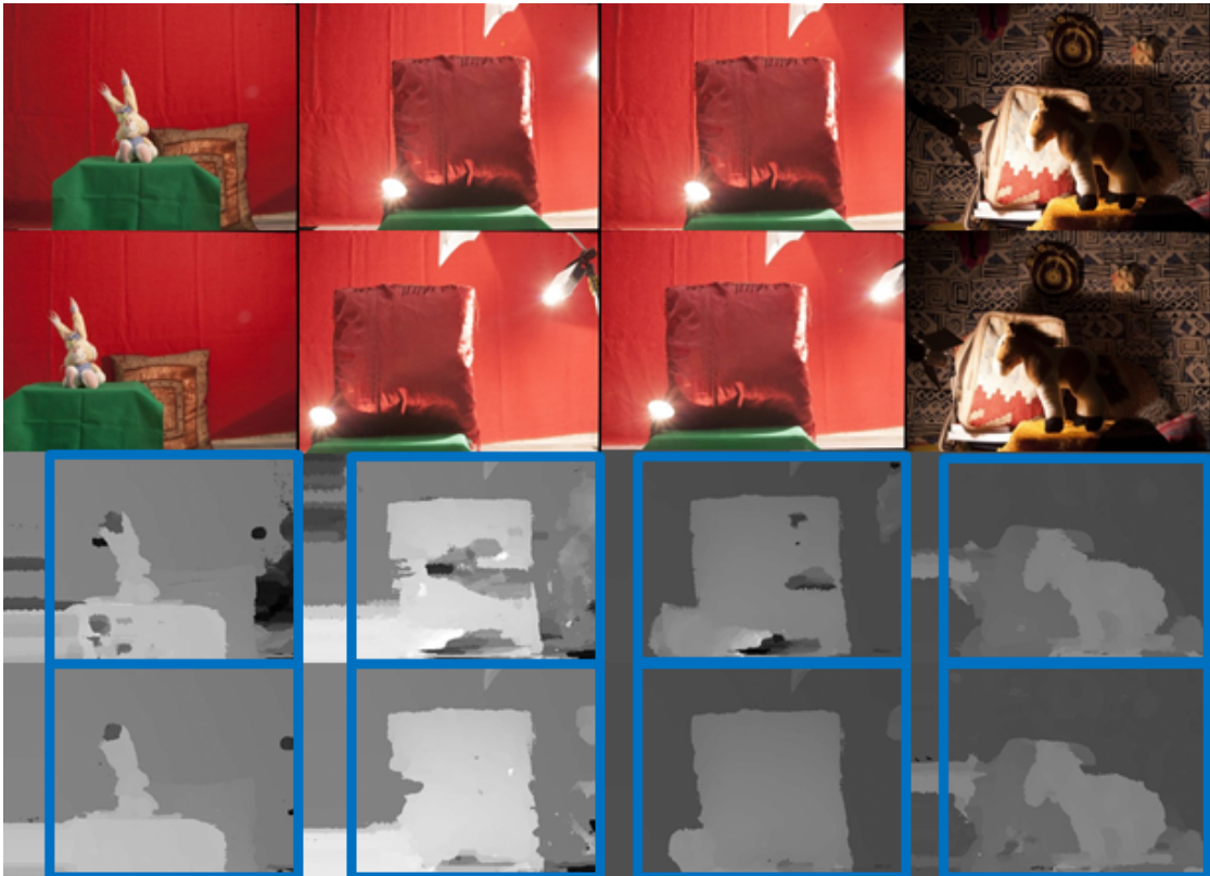
Figure 4.2: LDR-HDR stereo-matching comparison. Rows from top to bottom: left view, right view, LDR disparities, HDR disparities. Baselines, left to right: 150 mm, 150 mm, 75 mm, 75 mm.
