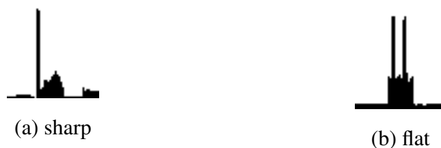
Figure 3.12: Flat (one peak) and sharp (two peaks) accidentals can be derived from the number of peaks in their vertical projection.
