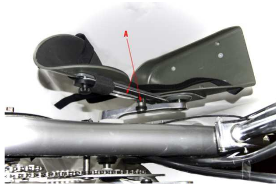
Figure 25 Position of the PES (A) on the left side, in driving direction, in end position.
