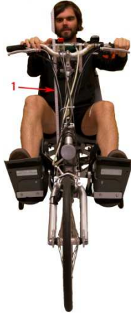
Figure 39 Cropped picture used to determine the wind contact surface. The picture includes a yardstick (1) to achieve a correlation between pixel number and surface area.
