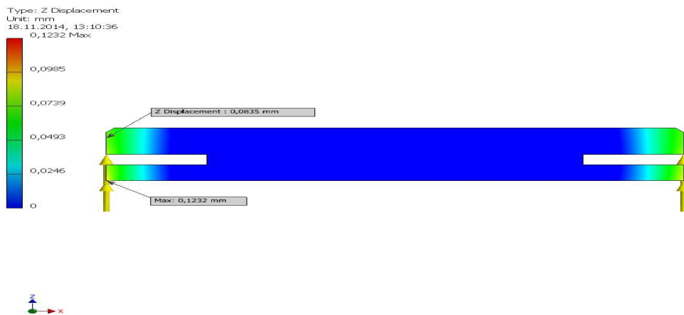
Figure 53 Analysis results of the horizontal beam, in vertical direction (Z-coordinate)
