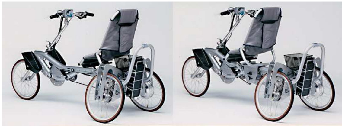
Figure 14 Picture of the bicycle in extension drive mode with the seat in end position (left side) and forward position (right side) (Pictures taken from [32])
