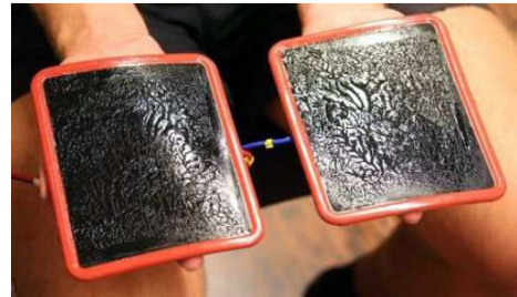
Figure 32 Safety electrodes with conductive layer pointing upward. On this picture electrode gel is used as conductive medium (Taken from [34])
