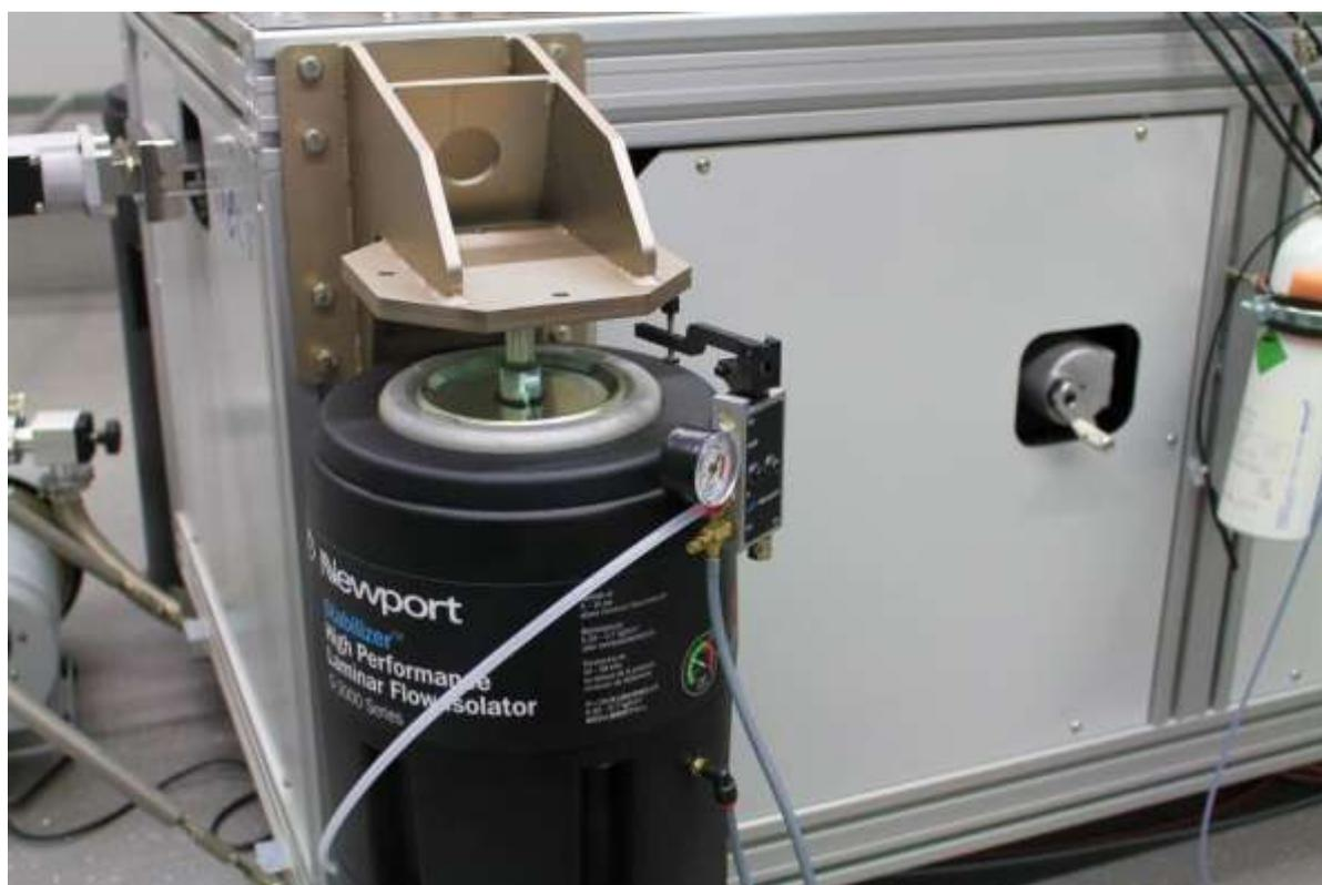
Fig. 2-46: Active anti-vibration system (air buffer) in our STM system.
