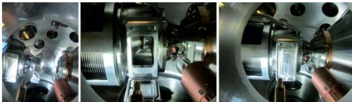
Fig. 2-28: HP-XPS cell. On the left side with open bayonet coupling to the analyzer, in the middle open sample inlet and on the right side ready for measurement.
