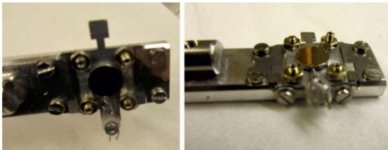
Fig. 3-65: Sample plate and transfer holder of the HP-XPS system. The transfer holder is used to move the sample from the load lock to the UHV chamber. Due to the arrangement of the vacuum chamber, transfer steps cannot be observed through a viewport, but could be observed by a camera.
