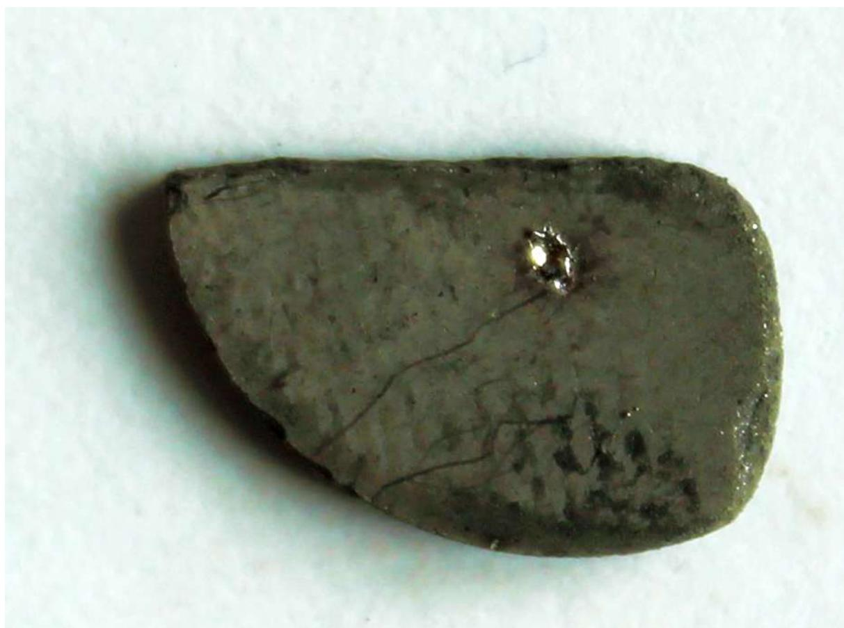
Fig. 4-27: Picture of the Pd<sub>2</sub>Zn pellet. The surface is rough and non-uniform, also some contaminations/enclaves in the bulk can be seen.
