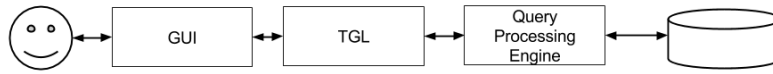
Figure 2.8: Graph database optimization via visual querying, simplified from [10] Fig. 2. GUI stands for Graphical User Interface and TGL is the TGL Translator, "[...] consisting of the query translation component and the result translation component".
