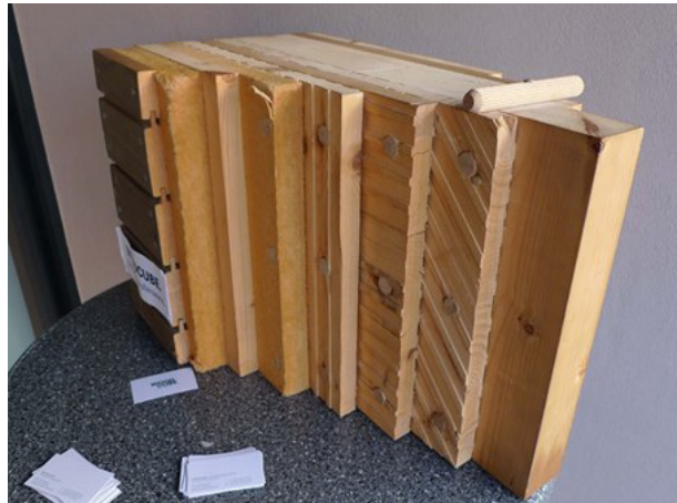
Fig.19: Wall composed entirely of timber products; Wood-cube project , IBA, 2013
