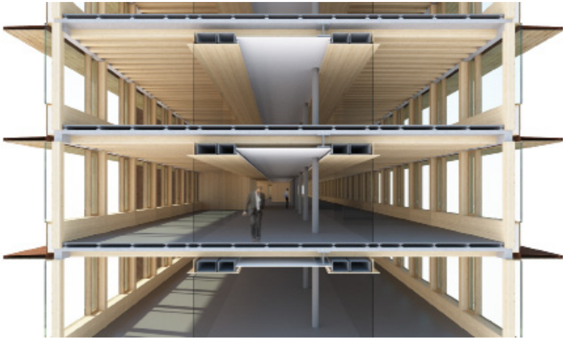
Fig.35: Life Cycle Tower, cross sections
