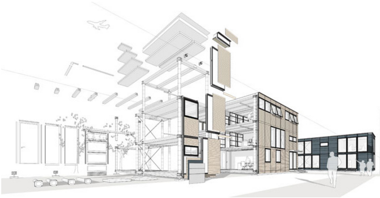
Fig.28: Building layers scheme by Lukas Lang
