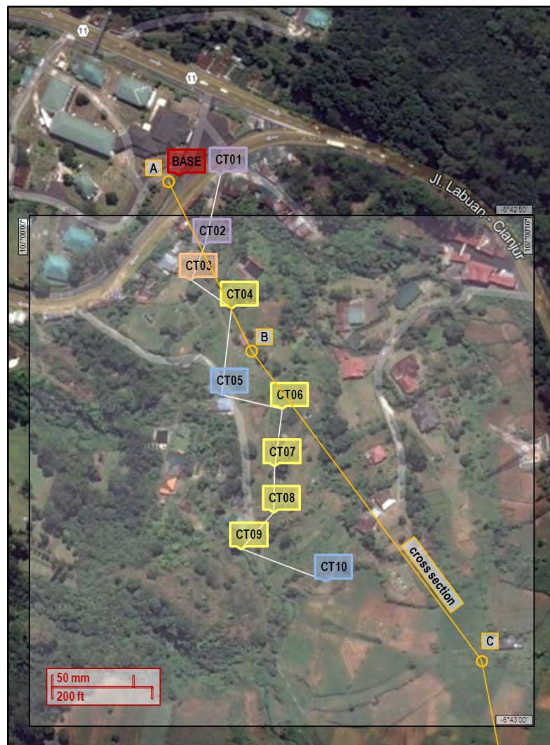
Figure 26: Observation points of the slope BASE = reference station; CT01 - CT10 = observation points
