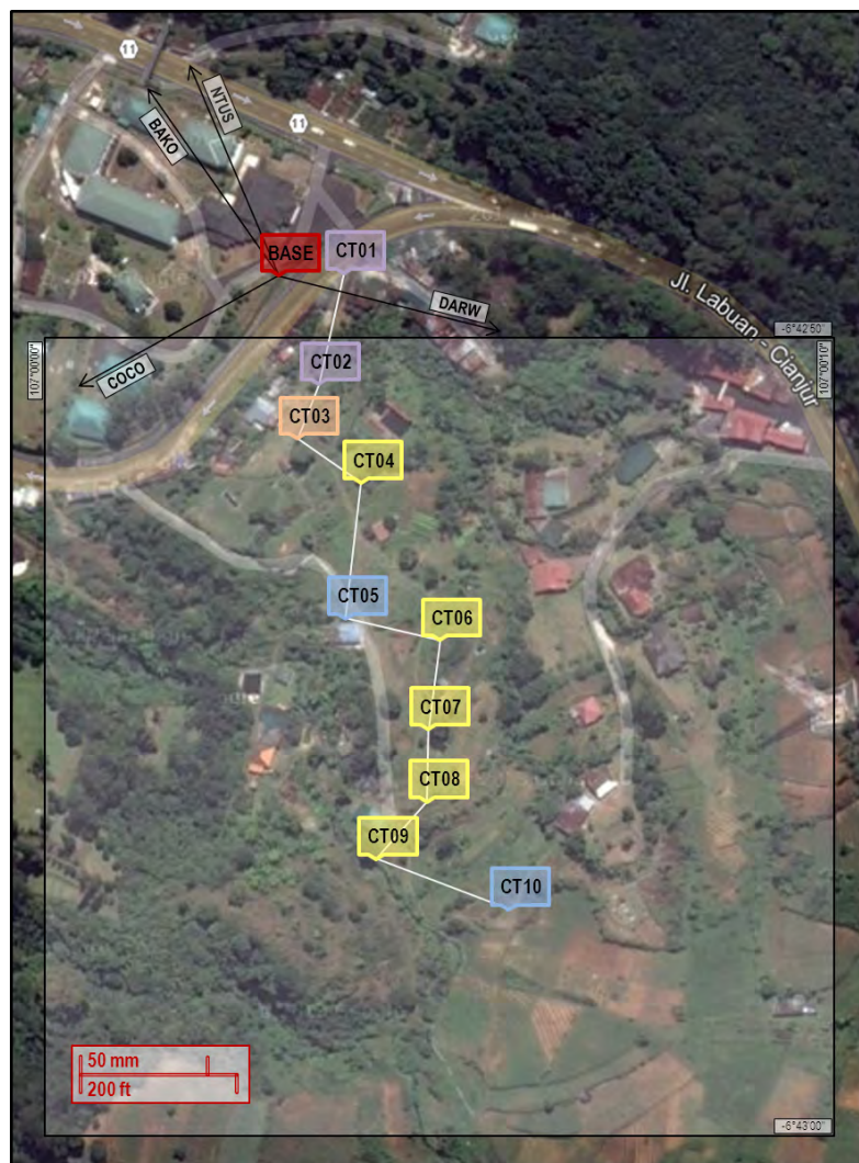
Figure 35: GPS data processing of BASE station BASE = reference station; CT01 - CT10 = observation points
