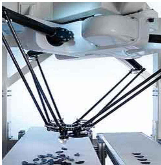
Abbildung 4.9 - High Speed Pick & Place Roboter Adept Quattro s650H/850 H , [26]
