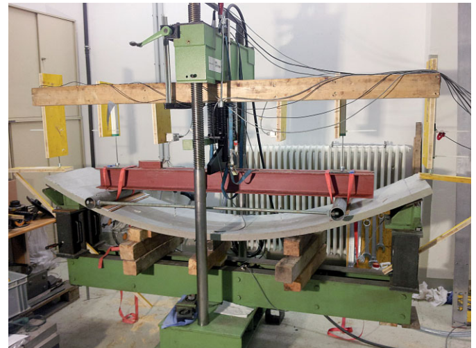
Fig. 8. Bending test with test specimen
