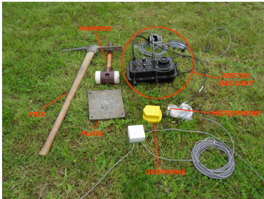
Figure 4.6.: Equipment used for the in-situ experiment at the Knödelhütte (Vienna)
