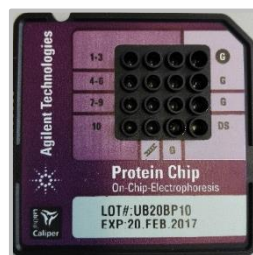
Figure 37: Chip used for protein analysis with the Agilent Bioanalyzer.
