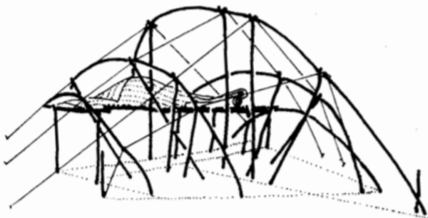
Fig. 199: Hadendowa (Beja), Sudan: system combining principles of armature and tent: bed is structurally integrated into the frame
