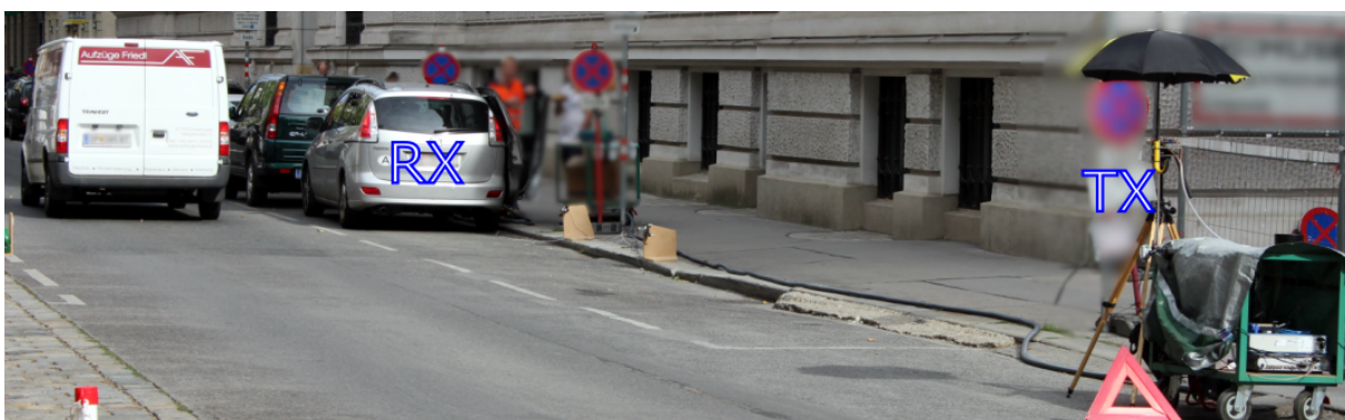
Figure 4.2: Measurement site. The TX and RX are static while urban street traffic is passing by. In this snapshot, the overtaking vehicle (white van) is at a bumper-to-bumper distance of approximately d = 6 \text{ m} .
