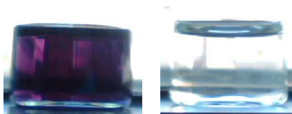
Figure 67. Solution of the violet product of the reaction with dimethoxy cyclohexadiene and tosyl chloride after dissolving and 30 min later. Complete discoloration occurred.
