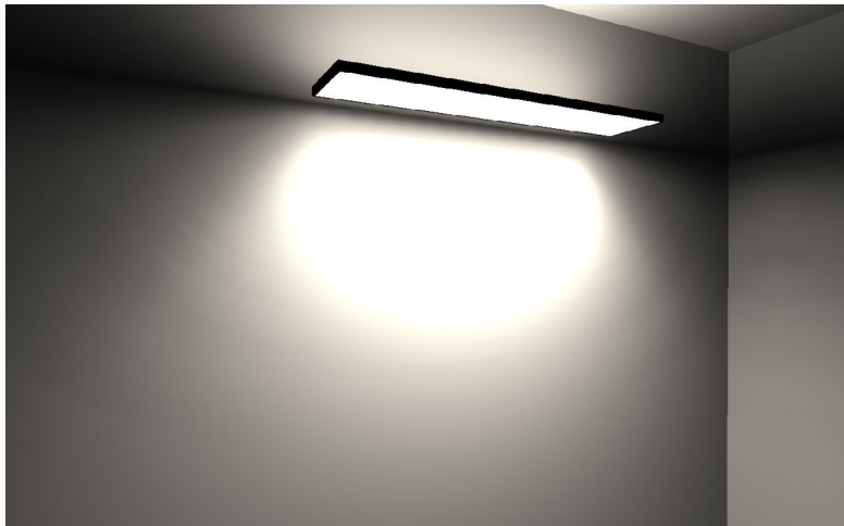
Figure 2.7: Relux approximates photometric light sources by using a collection of point lights. While this enables accurate previews, the interaction is not real time and requires the user to wait for a short time after something in the scene has changed.
