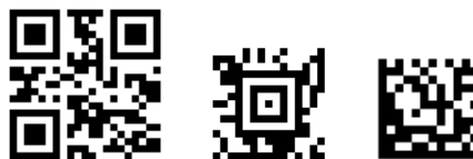
Figure 7.5: Popular 2D Barcodes with rectangular pixels: Quick Response, Aztec, Data Matrix
