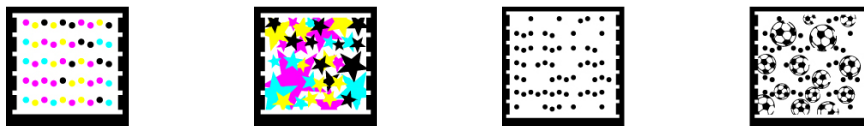
Figure 8.5: Microsoft Tag offers great customizability for concealing the data pattern but still needs a distinctive feature (i.e., a bulky border) for synchronization [208]
