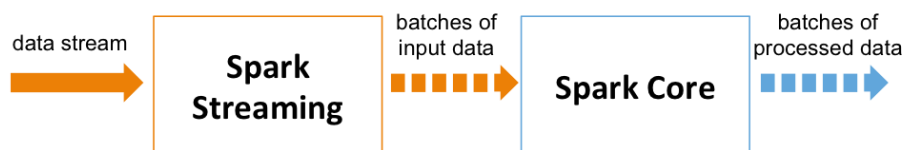
Figure 57: Mini-batch processing model of Spark Streaming.
