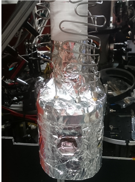
Figure 3.17.: The 4 K heat shield, attached to the 4 K base plate (see fig. 3.14) shields the experimental chamber from thermal radiation. The upper part of the base plate is wrapped in mylar and aluminium tape to prevent any exposed, less reflective copper parts.
