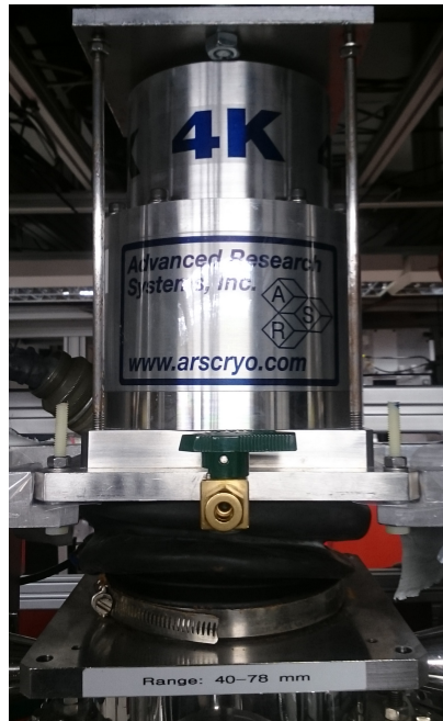
Figure 3.15.: The cryo head is on top of the cryostat and cools the experimental chamber via a cold finger. It is suspended from the ceiling and mechanically decoupled through a helium filled bellow, as seen in fig. 3.14.
