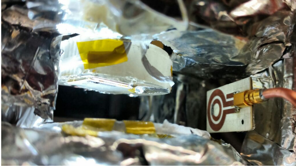
Figure 3.20.: Detailed view of the experimental chamber, which is the orange rectangle in fig. 3.14. The atomchip is suspended from the cold finger and the MW and RF antennas are in close proximity to it. The PCB with ring structures is the MW antenna with a resonance frequency of 6.83 GHz, to address the clock state. The RF antenna is a coil with 20 windings around the chip mounting. Its two connections going up can be seen in the forefront. A second back up RF antenna is on top of the V8 coil, which is, due to its greater distance to the chip less effective.
