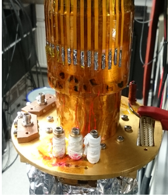
Figure 3.18.: Niobium titan wires painted with pink nail polish, to fix insulation. They are soldered to the YBCO HTSC bands and then routed, in tight contact to the base plate (see fig. 3.14), to the bobbins, where they are tightly wrapped around several times, for good heat anchoring.
