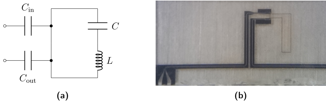
Figure 4.10.: (a) is a simplified schematic of an lumped element resonator with two capacitors to couple to feed lines. (b) shows a lumped element resonator design, to test in our bath cryostat. To the lower left the contact pads for the central conductor and ground plane are seen. Right of the center is a current loop, creating the inductance L , while left to it between the two capacitively coupled feed lines is the capacitance C , which is made of an array of conductor paths arranged like interlocking fingers.
