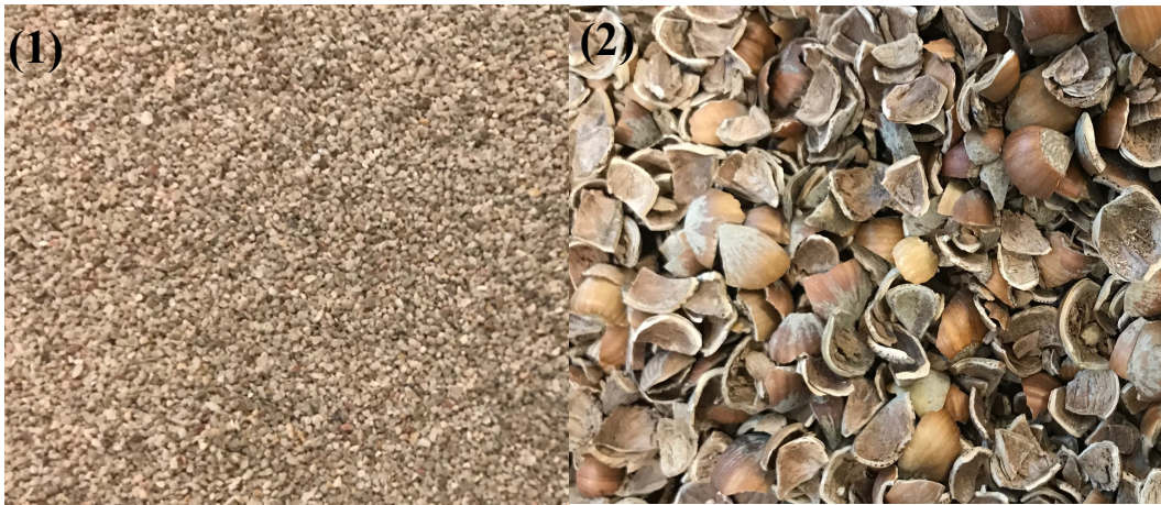
Figure 21: Limestone (1) and Hazelnut shells (2) which were used as bed material and fuel respectively.
