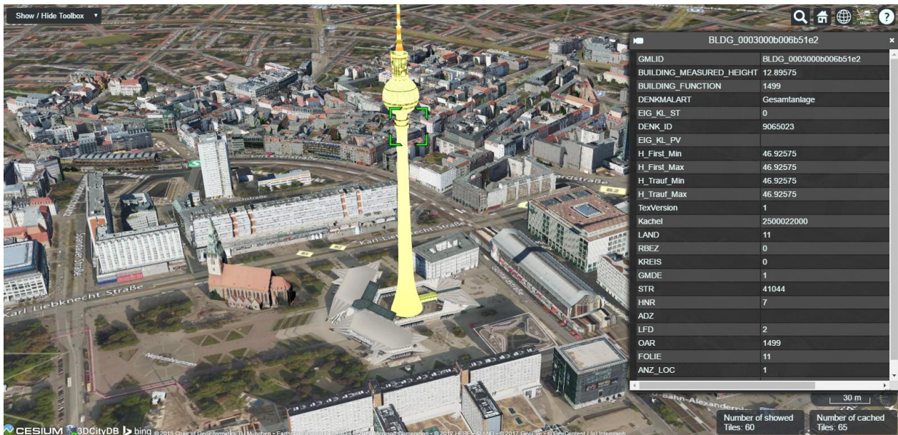
Figure 2.4: A semantic 3D city model of the German capital Berlin ( http://www.3dcitydb.org/3dcitydb/VisualizationBerlin/ , last access December 2016)
