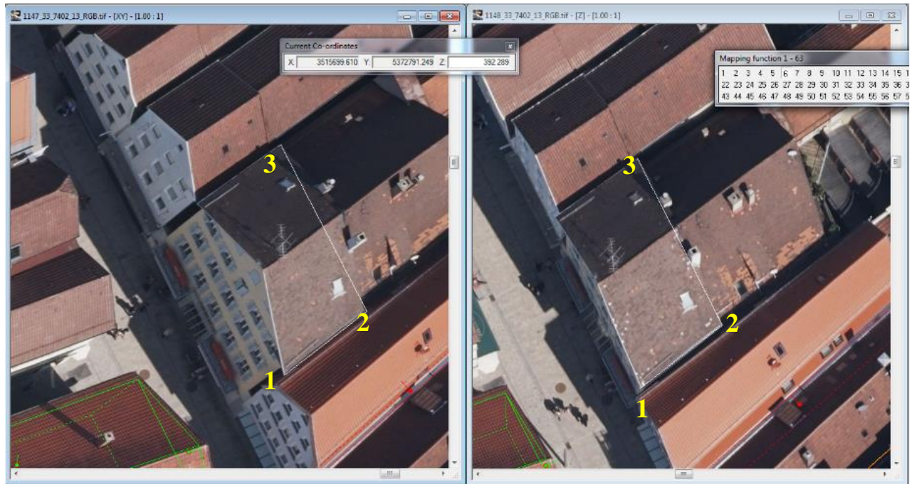
Figure 3.5: Measuring eave points of object with respect to constructional order
