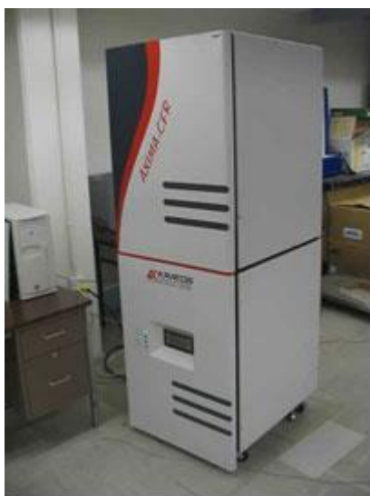
Figure 18: Axima CFRplus high vacuum MALDI mass spectrometer
