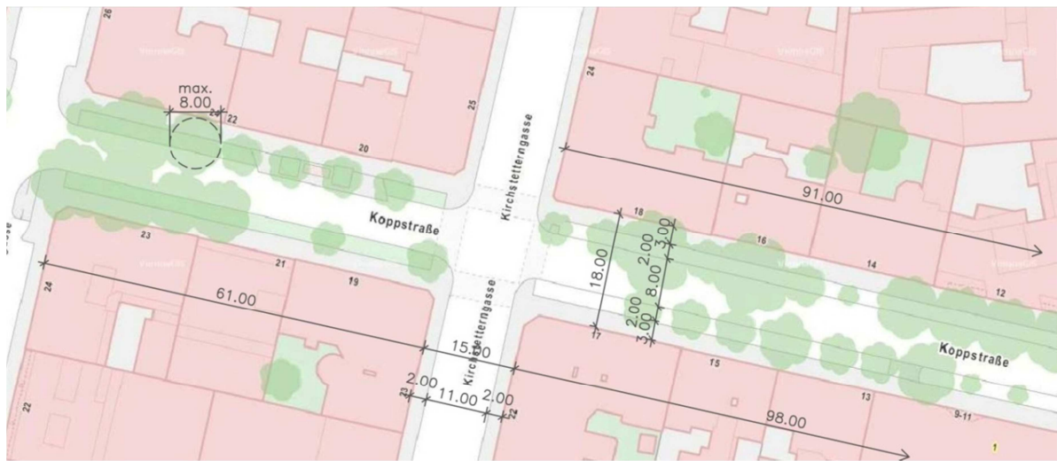
Figure 3.3 Dimensions Koppstrasse (in meters), crown diameter max. 8m
