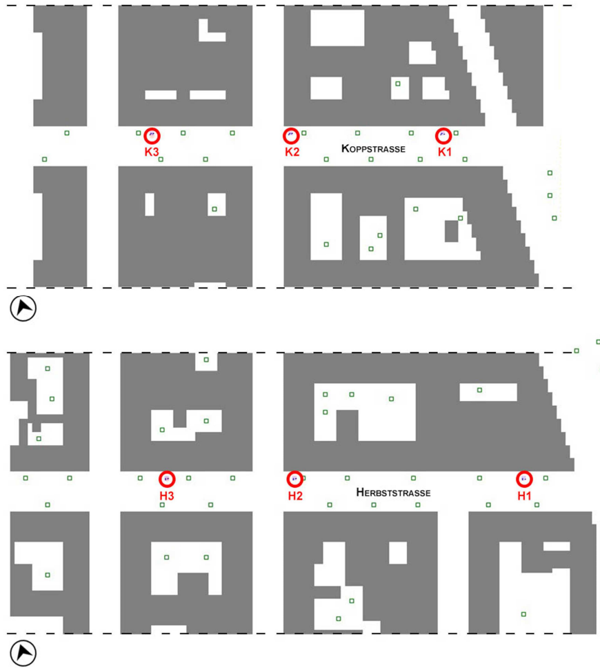
Figure 3.14 Top view of ENVI-met models in case C3 with the exact placement of trees at Herbststrasse and re-spaced trees at Koppstrasse
