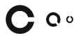
Fig. 2 The Landolt C is a standardized symbol to test visual acuity. It is a black ring on a white background with a gap on one side
