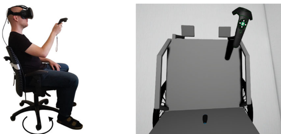
Fig. 6 Physical model of our wheelchair simulator (left) and virtual model of the wheelchair from the users perspective (looking down) (right)
