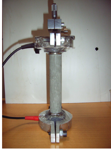
Figure B.2: Test setup consisting of the cylindrical cement specimen, the steel frame and the transducers covered by thin honey layers and food preservation foils
