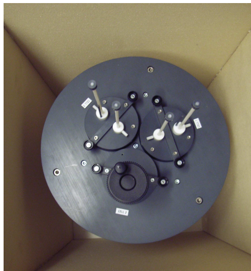
Figure C.1: Top view onto calorimeter ToniCal Trio type 7339 with three independent measuring cells
