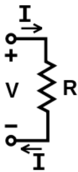
Fig. 43: Current flow through a resistor. Source: Gross & Roppel (2012)
