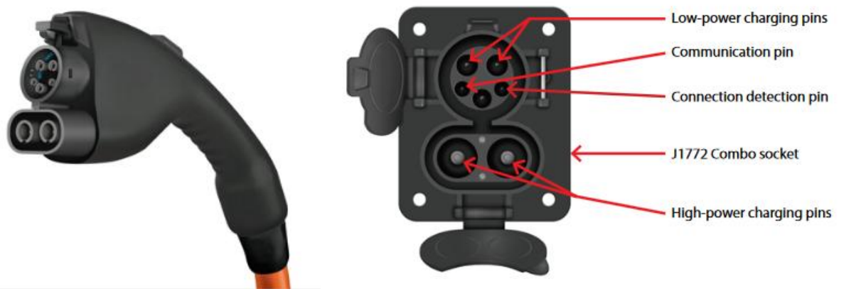
Figure 24: Fast Charging CCS Plug [left] and Socket [right] (Source: Hydro Quebec, 2015 )
