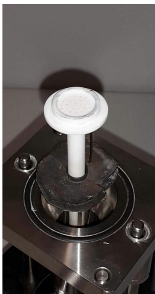
Figure S2b. Sample holder in the reaction chamber. The carrier gas passes the water vapour from the top through the sample.
