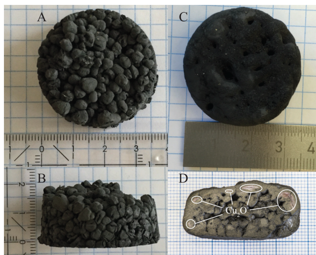
Figure 25. Sintering of the granulate material in the fixed-bed reactor: (A and B) top and side views after 1 cycle, (C) top view after 20 cycles, and (D) inside view of the material after 20 cycles.
