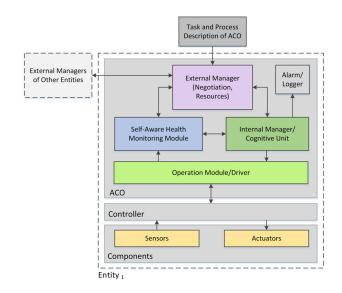
Fig. 1. The architecture of SAMBA depicting the structure of one Entity
