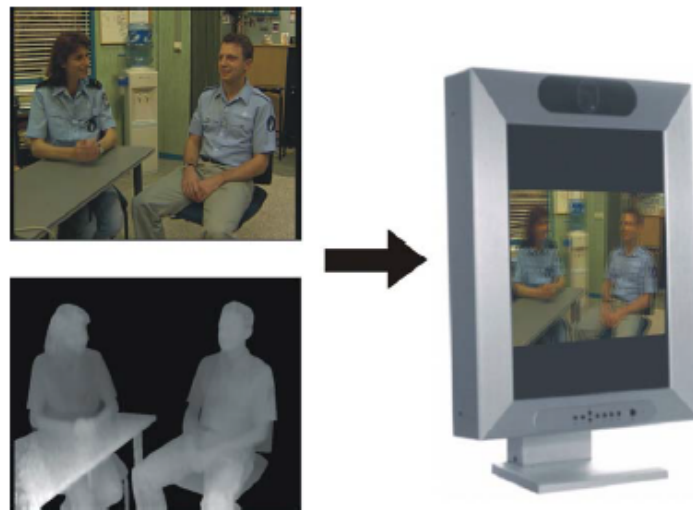
Figure 1.2: Illustration of video-plus-depth concept. A 2D color image with the corresponding depth map is used to create a stereoscopic image. A higher intensity value in the depth map means that the object is closer to the camera (Figure taken from [69]).
