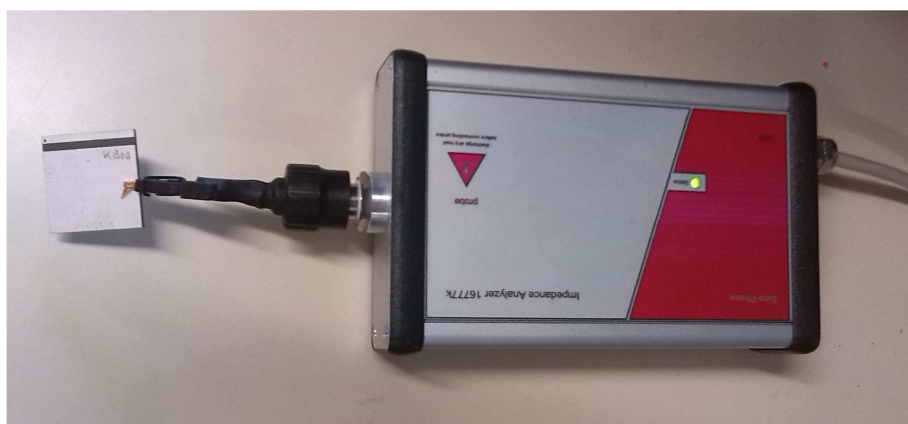
Figure 13: Picture of the Impedance Analyzer 16777k (SinePhase Instruments, Hinterbrühl, Austria) which is used to measure the conductance spectra of the PZTs.
