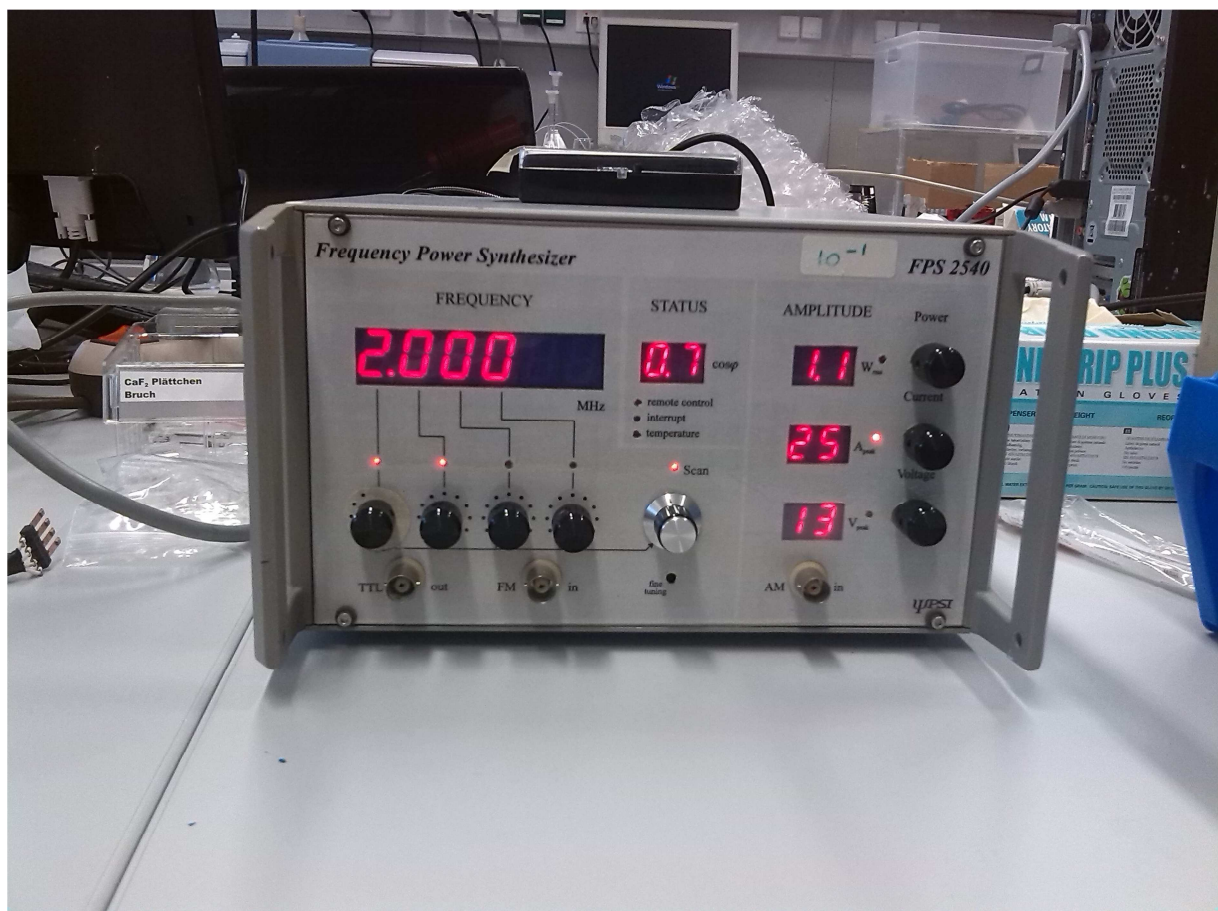
Figure 14: Picture of FPS2540 which is used to power the PZTs.
