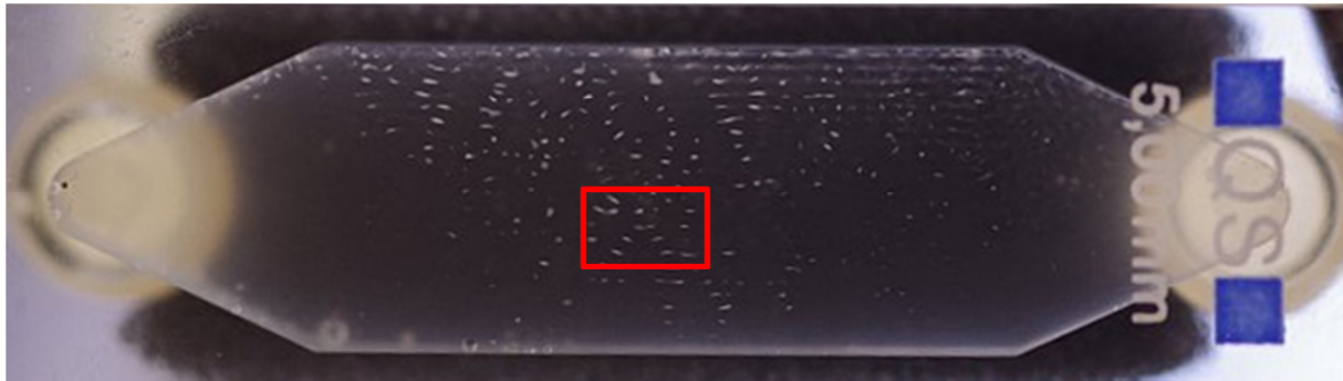
Figure 67: Photograph of cell1 driven at 2 MHz. Agglomerates of MCM-41 particles are clearly visible.
