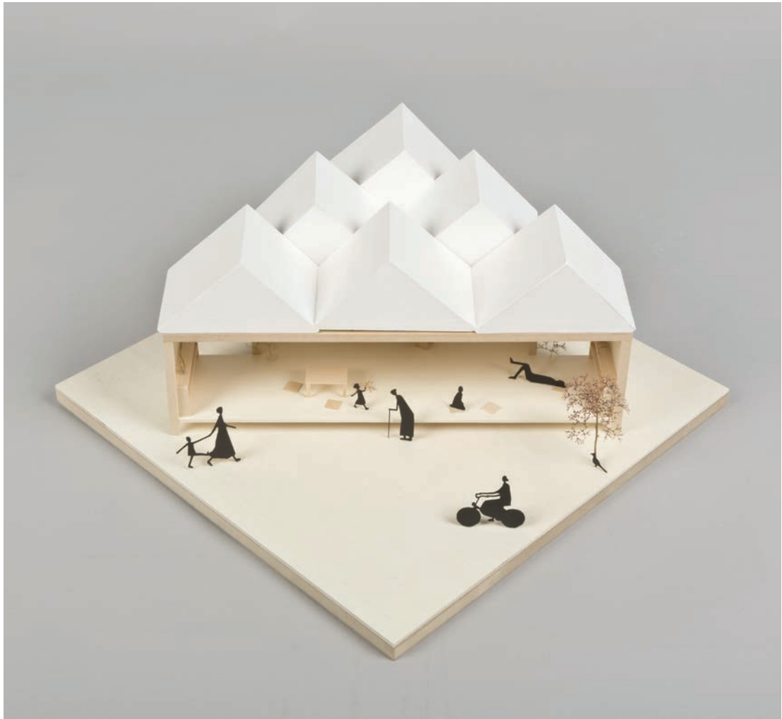
Img. 62: Pocket House Step III model, scale 1:33/ roof scape of the new structure
