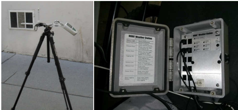
Figure 26: Mobile measurement equipment for areas B through E (left); detail of the weather station control panel (right)
