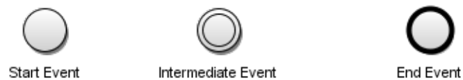
Figure 2.2: Representation of basic types of Events taken from tool Yaoqiang BPMN Editor 2.2
