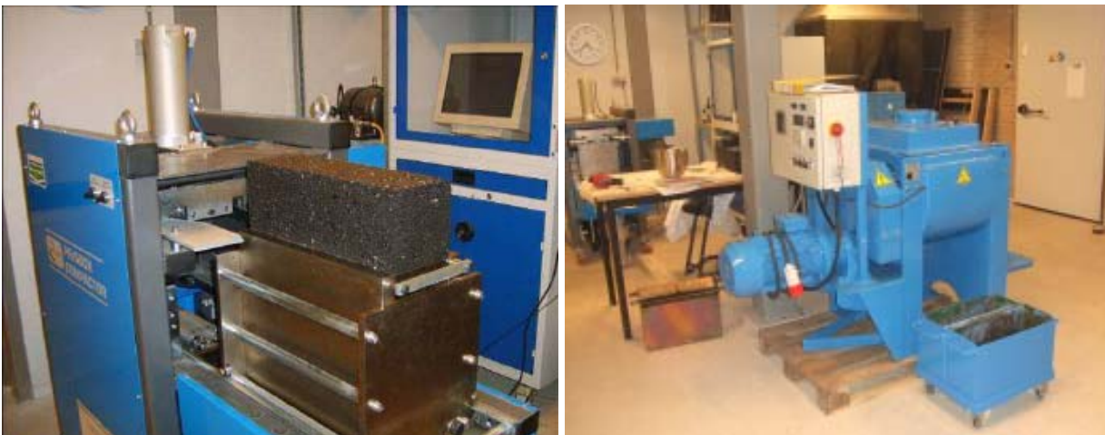
Abb. 4.7.1 Shear Press Box Compactor [TU DELFT]
