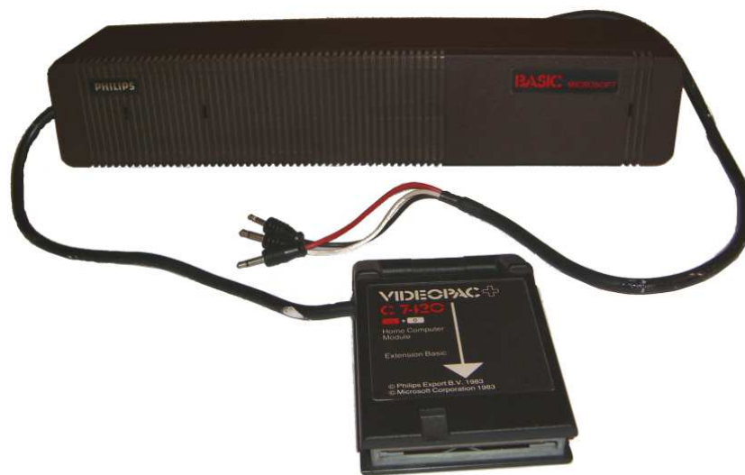
Figure 7.2: Philips Videopac+ C7420 Home computer cartridge: Cartridge that plugs into the system in front, connected to the main case that holds the additional CPU and memory in the back. The connectors for loading/saving data to an audio system (red, white and black cables for microphone, headphones and remote control) are attached to the main case.
