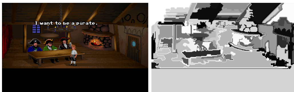
Figure 2.8: Screenshot of original DOS-Version of "The Secret of Monkey Island" (left). Significant areas in the same screenshot as a result of binarization and segmentation are shown on the right.
