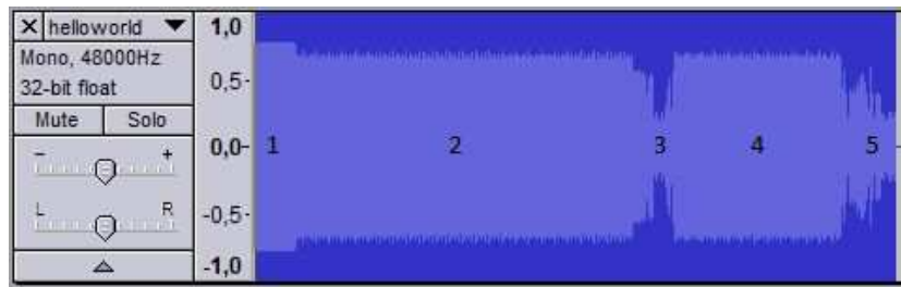
Figure 7.3: Waveform of “Hello World” BASIC program (1: initial 6 kHz lead-in tone; 2: 256 x 0xFF as start of file-signature; 3: file header; 4: 128 x 0xFF as header/data separator; 5: data block)
