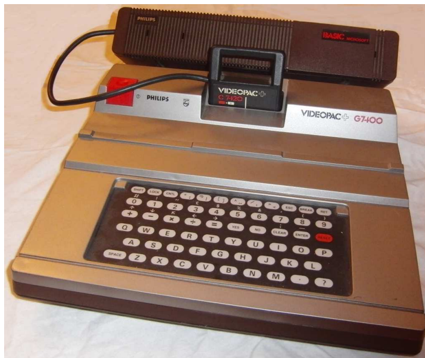
Figure 7.9: Philips Videopac+ G7400 with plugged in Philips C7420 Home Computer cartridge.
