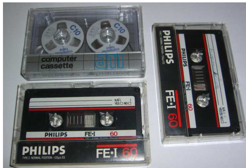
Figure 7.7: Tapes used for evaluation of migration tool, left upper corner C10 computer cassette, left lower and right Philips FE-I 60 normal position audio tapes.
