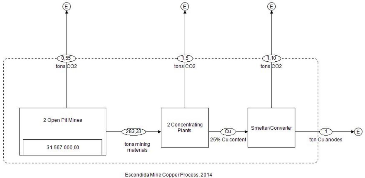
The material flow analysis for the Escondida Mine shows the amount of material needed in order to produce one tonne of copper anodes, while also showing the amount of carbond ioxide produced. This diagram does not show mass balances, but is instead an unbalanced flow diagram.
