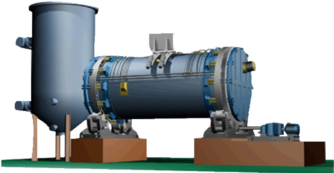
An example of an anode furnace (Kopar, 2010)
