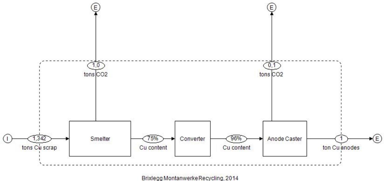
The material flow analysis for Brixlegg shows the amount of copper scrap needed to produce one tonne of copper anodes and the amount of the resulting carbon dioxide emissions. This is not meant to show mass balances but instead show an unbalanced flow diagram.
