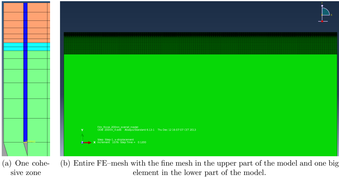
Figure 2.2: Entire FE-mesh with a detail from one cohesive zone.
