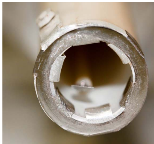
Figure 3.53: Sealing ring in the open part of the tubular reactor.
