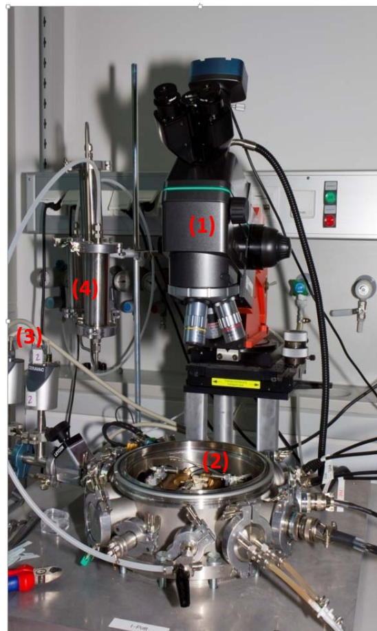
Figure 3.12: Setup for electrochemical characterization with microscope (1), chamber with heating stage (2), pressure gauges (3) and humidifier (4).
