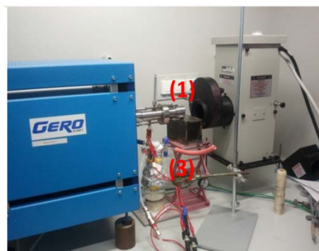
Figure 3.18: Setup with a light source by using a 1000 watts xenon arc lamp.
