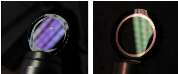
Figure 5.5 Damaged spots on pellicle outcouplers.
