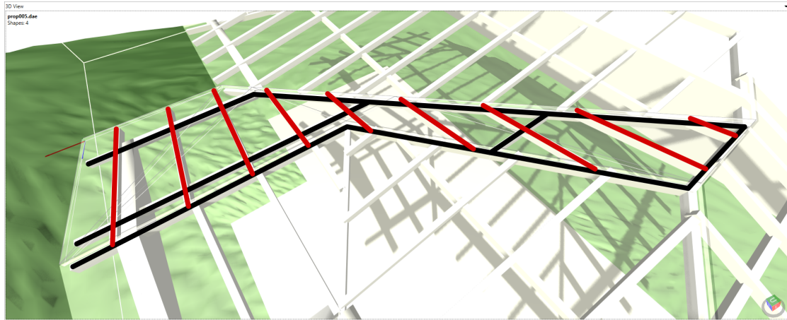
Figure 3.16: Complex additional roof geometries. The purlins are highlighted in black for one roof part and the rafters are colored red.
