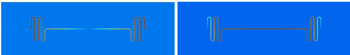
Figure 5.2: Left: Simulated electric field strength on a resonator surface with design 111, blue (lowest) to red (highest), arbitrary units. Right: Simulated magnetic flux density on a resonator surface with design 111, blue (lowest) to red (highest), field scale in arbitrary units.
