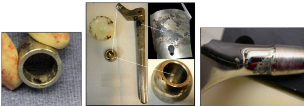
Fig.1: Images of parts of a hip-joint implant, which was affected by a corrosion process.
