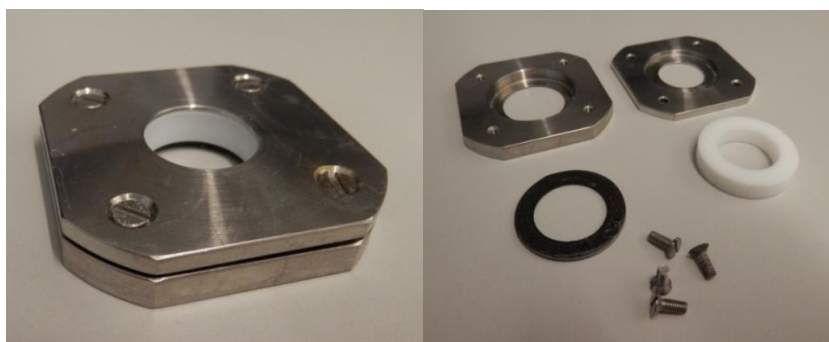
Fig. 72: Image of the sample holder: left – in the assembled condition, right – in the disassembled condition.
