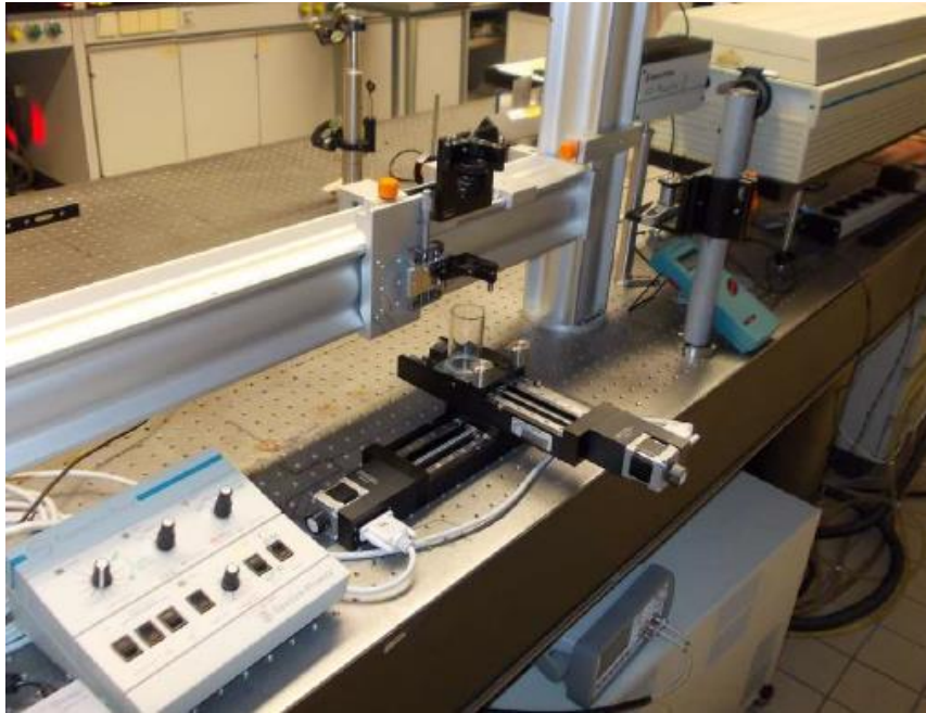
Figure 36: experimental setup for laser ablation in liquid (University of Vienna) 2
