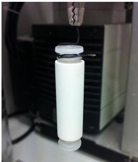
**Figure 19: Set up for dipping of tubular slipcast supports**
