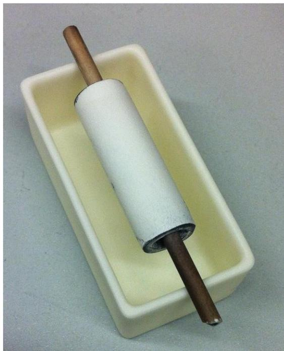
**Figure 21: Arrangement for pyrolysis of tubular coated supports without touching the crucible**
