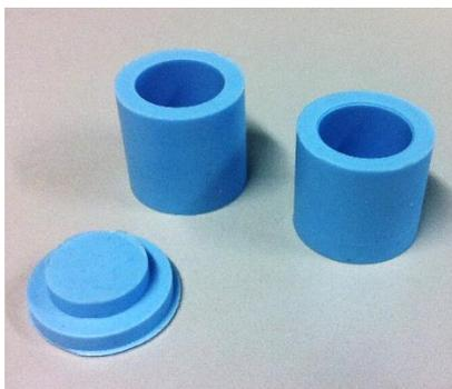
**Figure 13: Silicone molds used for casting of the PDC supports**
