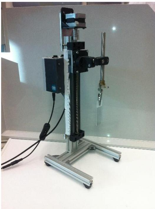
**Figure 17: Dip coater used for the experiments**
