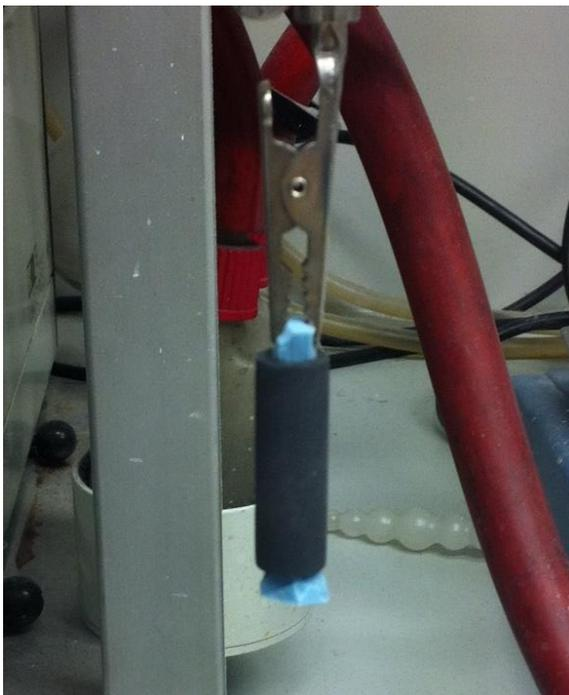
**Figure 20: Set up for dipping of tubular PDC-supports**
