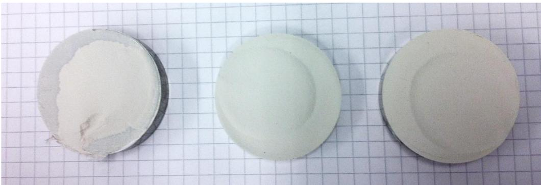
**Figure 16: Actual warm pressed sample in the middle, top and lower punch on the sides**
